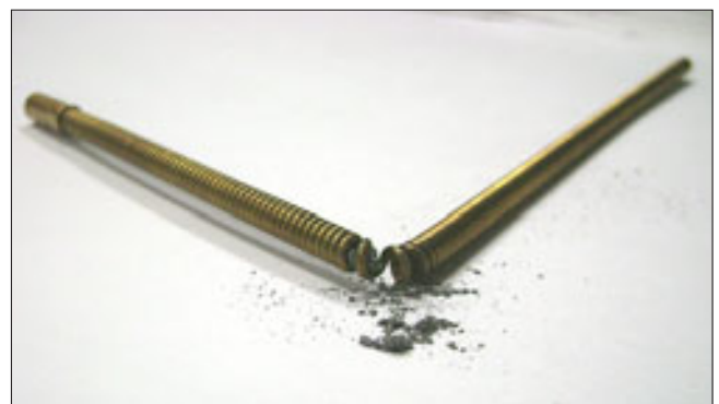
Above: Showing clogged liner with aluminium particles
